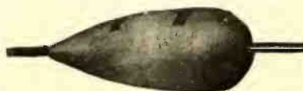
Special Wireless Telephone Dynamo Recently Developed for Use on Aircraft. It Combines Two Dynamos, One Giving 6 Volts and the Other 1500 Volts, For An Oscillation.
