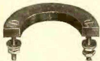
B Battery Potentiometer Unit
