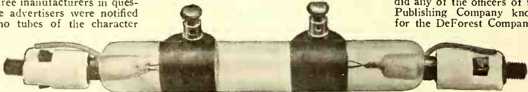
The Tigerman Detecto-Amplifier which Uses Two Filaments and Two Cold Plates in an Evacuated Tube. It Also Uses Two Outside Members as Shown.
